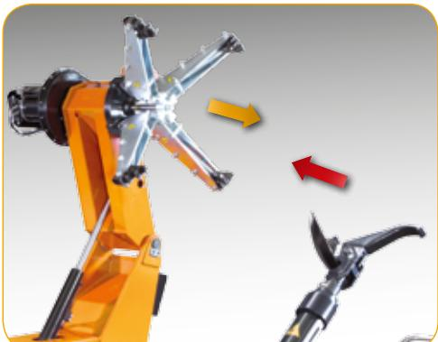
**EN** • Independent movements between self-centring clamp and tool arm.
