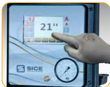
**EN** → • **Program** wheel dimension in inches (13" - 32") and the best radial wheel positioning on the automatic "Revolver".
