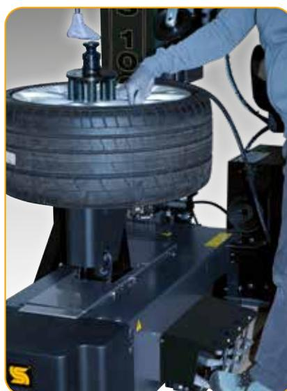
**EN** → • **Insert** the handle with the clamping cone
