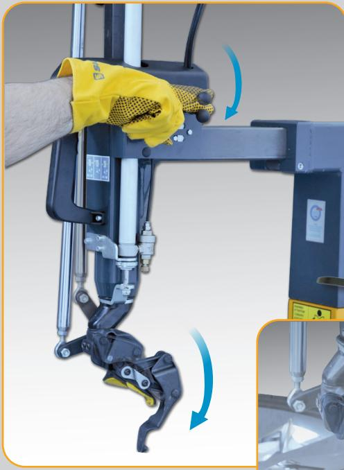
**EN** • “**LEVERLESS**” DEMOUNTING: fast and easy leverless tool head, a simple switch activates the “leverless” system.
