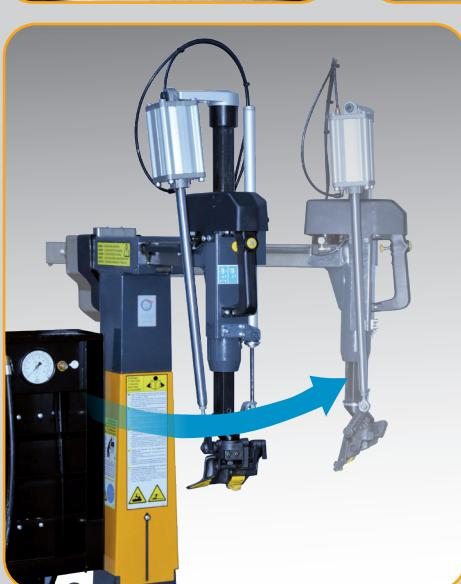
**EN** • Pneumatically rotated post (**patented**). Significantly reduces space requirements.
