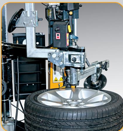
**EN** • **“CONTACTLESS” mounting:** the PT, bead pressing device, allows tyre mounting on any wheel without the aid of clamps.
